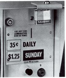
SECURE: Constructed with a single case-hardened post shackle, this Master Lock padlock eliminates the part of a lock most susceptible to attack – the loop of the shackle. Rekeyable padlock is finding wide vending application.
