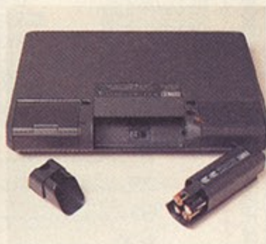
• The battery pack takes 8 standard batteries. A NiCad pack is also available
