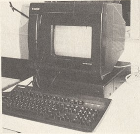
• Canon's navigator: fax, PC, printer, modem and phone all in one package. It even has a touch-screen
