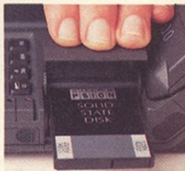
• The 'disk' drive takes solid state disks – battery backed to conserve data
