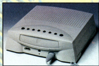
The Pippin measures 3.2 inches high, 10.4 inches wide, and 10.6 inches long. Slightly larger than a Saturn, it weighs 8 pounds.
