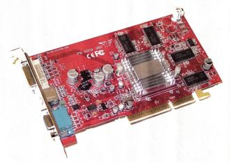
reference design, and it also means that the card doesn't need an additional power connector, unlike so many designs that we see these days.
