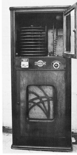
This prime J.P. Seeburg machine's cabinet holds an AC/DC electric converter and a turntable for each disk. Play setting: 3 for 10 cents.
