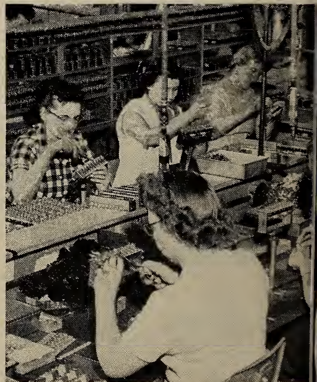
One-button play, much wanted feature of all AMI phonographs, begins here with the assembly of the selector button banks. Highly trained personnel, usually women, who excel in manual dexterity, are especially selected for this precise assembly operation.
