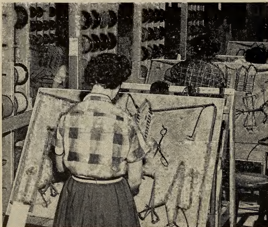
The complex wiring of the modern juke box gets its start with this ingenious new arrangement of spools and harness boards. Here deft operators tie hundreds of feet of vari-colored wires into compact networks that transmit electrical impulse with unerring accuracy.
