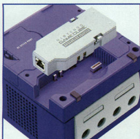
■ This gray, modular broadband adapter snaps easily into one of the three expansion ports located on Gamecube's underside
