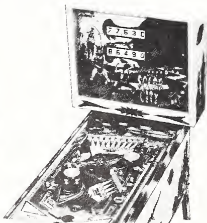
GOTTLIEB 'SOLAR CITY' — A 2-player pingame with plenty of playfield action. Fifteen drop targets geared to increase bonus value; four flippers; rollovers for extra ball and special, etc. Futuristic graphics are eyeappealing. (2/26/77).
