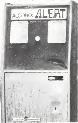
ALCOHOL 'ALERT' A coin-operated breath testing device manufactured by Alcohol Countermeasures Inc. of Port Huron, Mich. Unit is designed for 25¢ pricing but is adaptable to $1.00 per test. (1/29/77).
