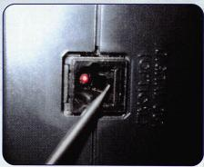
Nearly every modern surround receiver will have an optical input as shown on the left. The two RCA digital inputs to the left of the optical are known as coaxial or electrical. and the PS2 does not support these. On the right, a peek inside the PS2's optical output.
