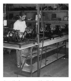
Greg Clevinger assembles the base mechanisms used in the Fun Riders line.
