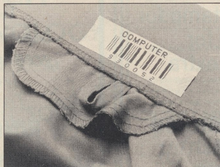
Yet another bar code application - this one has been woven into clothing.
