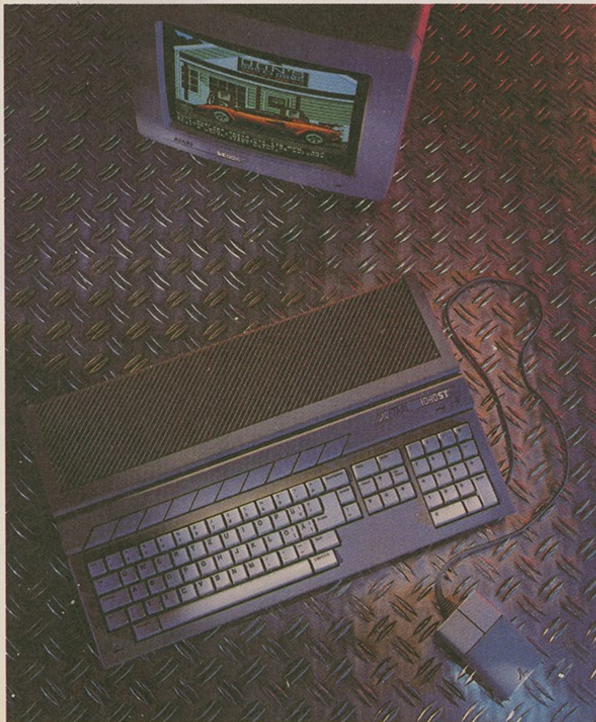
• The STE: in appearance rather similar to the 1040, note the conspicuous 'E' on the nameplate
