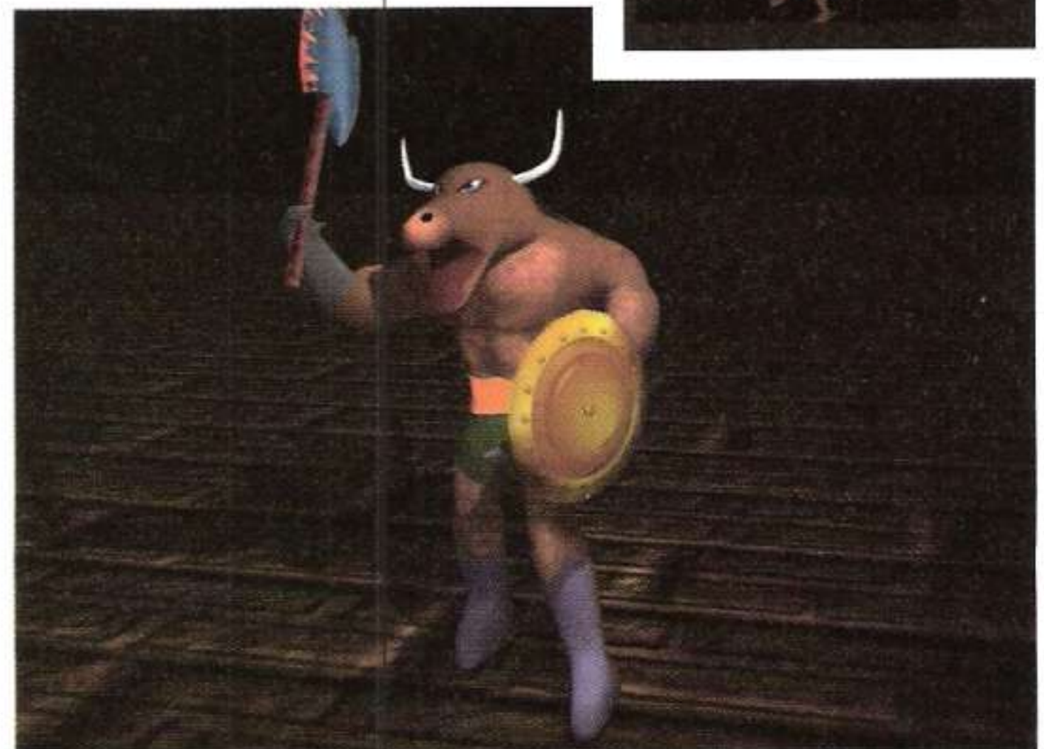
Note the absence of textures on the characters. Not only does this speed rendering, it enables developers to use more polygons per character. An additional advantage is that characters stand out against textured objects
