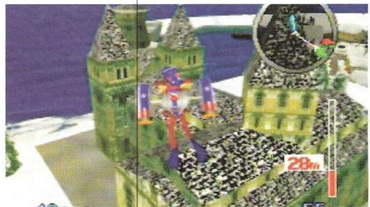
Bilinear filtering and anti-aliasing: textures are smooth and show little or no pixelation, while edges of objects show none of those nasty "jaggies"
