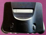
The Nintendo 64, shifting over 500Mb of data per second, doesn't segment RAM, meaning memory restrictions are less of a problem
