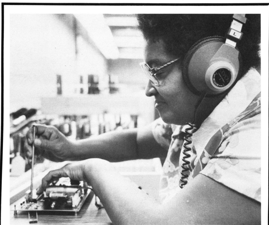
How does Williams Electronics ensure that its industry-renowned electronic sounds gurgle, beep, and plink just right? With a customized test fixture and a special pair of earphones, of course, as illustrated here by a Williams employee at the firm's Chicago plant as she makes a final check on the sounds component.
