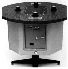
state 12-inch television monitor are at the heart of the Fascination 500 and the screen is covered with quarter-inch commercial grade plate glass to provide breakage resistance and long-life. The glass is bronze smoked to reduce glare and the entire electonic system is mounted in a cast iron base with self-leveling shock absorbers.
