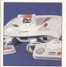
Availability: most major high street retailers Dimensions (mm): 255 x 184 x 54 Weight: 600g Memory: 64K Processor: 4MHz Z80A Sound: stereo, three-channel programmable AY-3-8912 sound generator Maximum onscreen colours: 32 Palette: 4096 Resolution: 160 x 200 Cartridge capacity: 128K Software: one title, ten-plus in production
