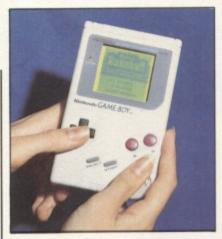
Availability: certain high street chains Dimensions (mm): 146 x 88 x 32 Weight: 320g Memory: 8K Processor: ???? 6502 Sound: stereo, three channels Maximum onscreen colours: n/a (black and white only) Palette: n/a Resolution: 160 x 144 Cartridge capacity: ???? Software: 50-plus, numerous new releases
