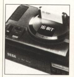
Availability: certain high street chains Dimensions (mm): 280 x 212 x 65 Weight: 800g Memory: 74K main plus 64K video Processor: 8MHz 68000, plus 4MHz Z80 for downward compatibility Sound: stereo, 12-voice custom FM chip Maximum onscreen colours: 64 Palette: 512 Resolution: 320 x 224 Cartridge capacity: ??????? Software: 30-plus, many in development
